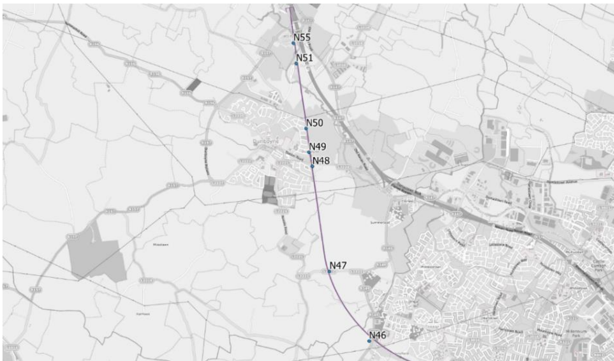
Figure 14-3 Noise & Vibration Survey Locations Zone D
